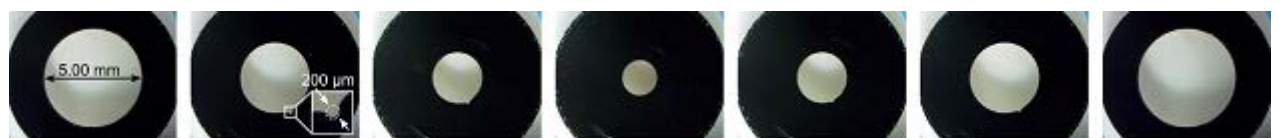
Fig. 12.30. Photographs of the actuation of a microiris chip, demonstrating reversible aperture tuning.
